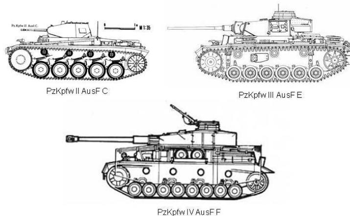
**Figure 11. Basic German tank thread.** The PzKpfw II, at less than 9 tons and armed with a 20mm gun, was by 1943 reduced to a light reconnaissance role as the *Luchs* (Lynx). The PzKpfw III, which weighed in at 23 tons with a 37mm gun, was rarely seen in the East and reduced to a backup role elsewhere. The PzKpfw IV in various modifications lasted the entire war.
