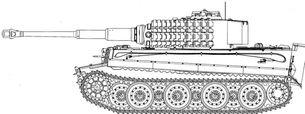
**Figure 13. The Tiger I.** This is officially *PzKpfw VI Ausf. H*. This version was the result of a competition of prototypes designed by Henschel and Krupp; the "H" indicates Henschel. The Krupp/Porsche consortium produced a number of chassis for their tank that were converted to heavily armored guns (the
