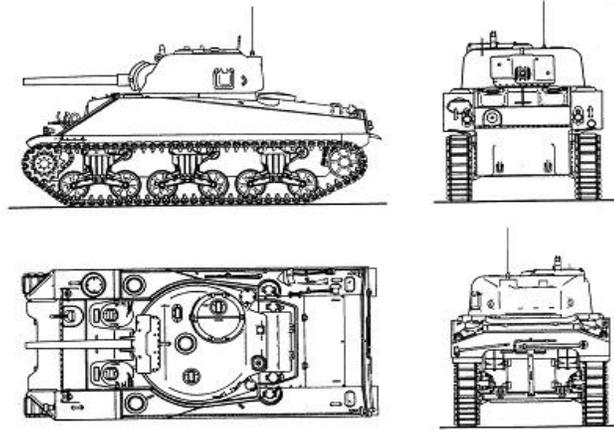
**Figure 1. A tank.** The M4 series was widely produced in WWII; most examples were typical tanks like the one above, but the carriage was modified for use in other applications. The original M4 was easy to produce, using a gasoline engine and a tractor-style vertical volute spring suspension (late models used a horizontal volute spring system, HVSS, which provided a smoother ride).
