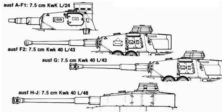
**Figure 12. Evolution of the PzKpfw IV.** The Pz IV was the heaviest tank in Germany's fleet in 1940, and began its active combat with a short 75mm L24 That eventually grew to an L48. There was a drive to add appliqué and bolt-on armor plates as well.
