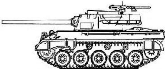
**Tank destroyer, M18:** This model was produced in 43-44 until production of the M36 was established. The M18 did not use a Sherman chassis, but a unique design with torsion bar suspension and a 450 hp aircraft radial engine, a combination that allowed a road speed of 60mph. The main gun was the 76mm that was being developed for newer Sherman models.
