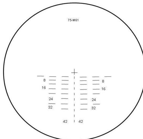
**Figure 5. Gunner's sight reticule for the M4's 75mm gun.** If the target is within boresight range (600m or less), the gunner can simply place the center cross on the target and blaze away. At a longer range, the gunner can simply elevate the gun (which will move the center cross up) until the target is on the dashed vertical line close to the estimated range. If the target is moving, the gunner has to respond to the
